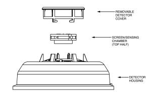
Figure 5. Removing Screen/Sensing Chamber
